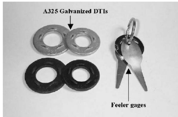
Figure 3-2. Direct Tension Indicators and Feeler Gages
