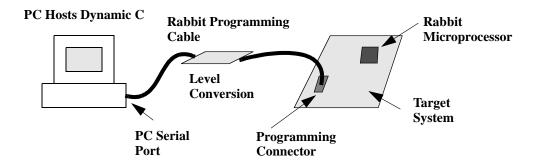
Figure 1. The Rabbit Microprocessor and Dynamic C
