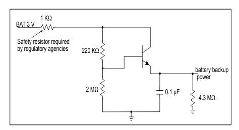
Figure 3. Clock Oscillator Regulator Circuit
