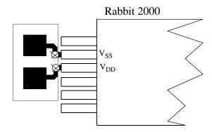
Figure 7. Decoupling capacitor placement and layout.
