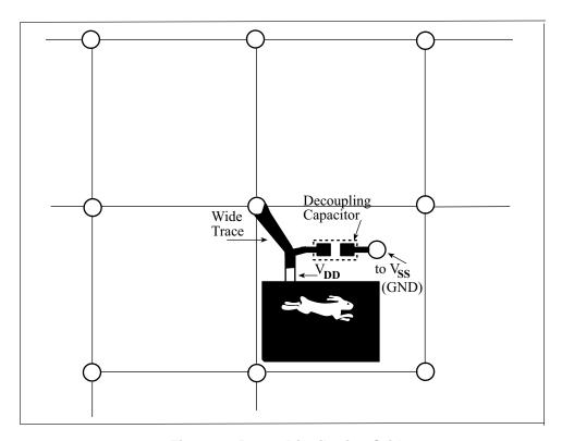
Figure 8. Power Distribution Grid
