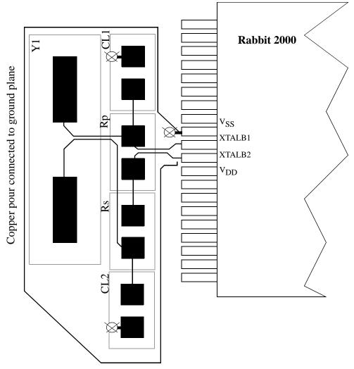
Figure 6. Avoid coupling the clock to other lines.
