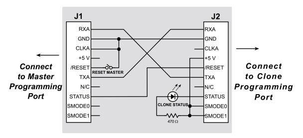
Figure 12. Cloning Board
