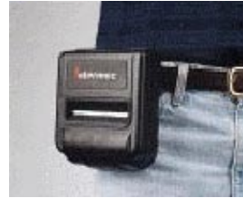
...Then use Bluetooth to send the information to a printer worn on the hip to make a receipt.
